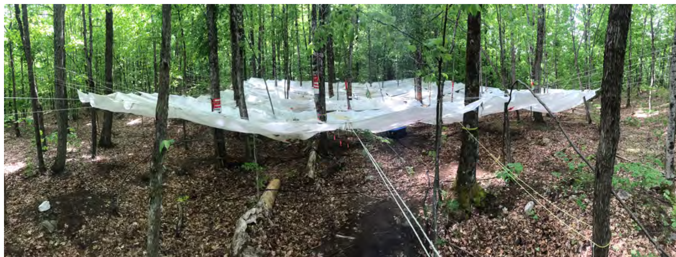
Throughfall-exclusion treatment using semi-transparent tarpaulins.
