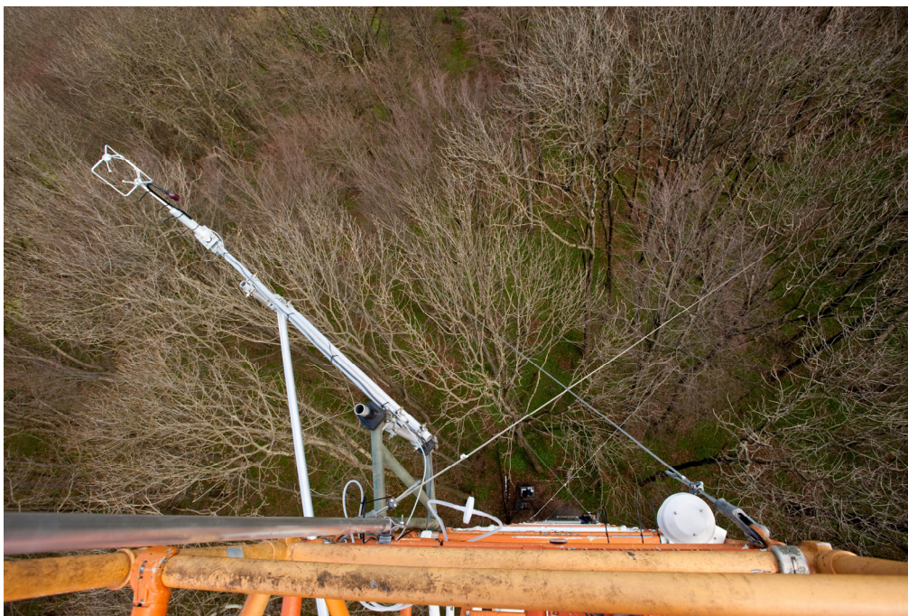
Figure 2 Eddy covariance measurement system at the Hainich tower, Germany (this figure can be used reproduced in the context of this paper. Please include image credit to © Max Planck Institute for Biogeochemistry, Jena).
