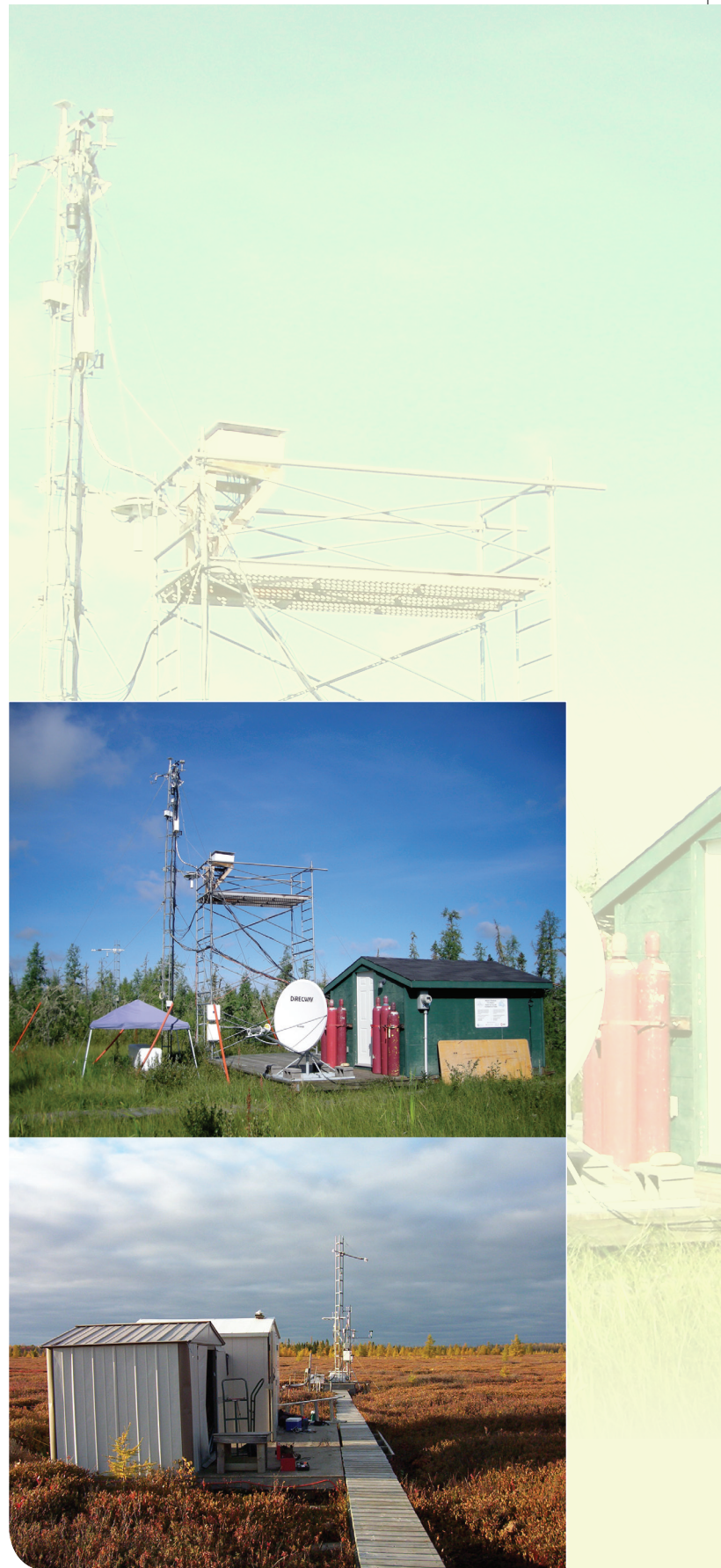
Figure 2. Western Peatland (top) and Eastern Peatland (bottom) Flux Station eddy covariance towers.
